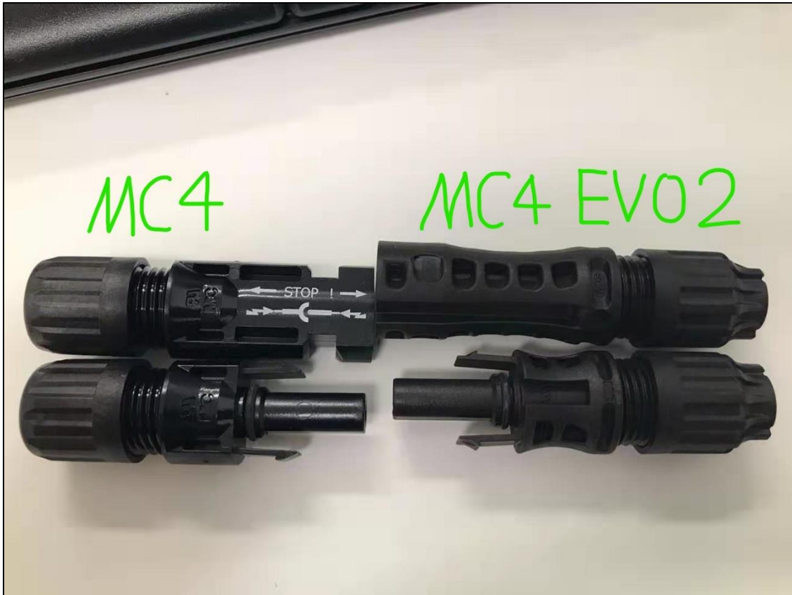
Figure 1. Physical appearance difference between MC4 and MC4 EVO2
