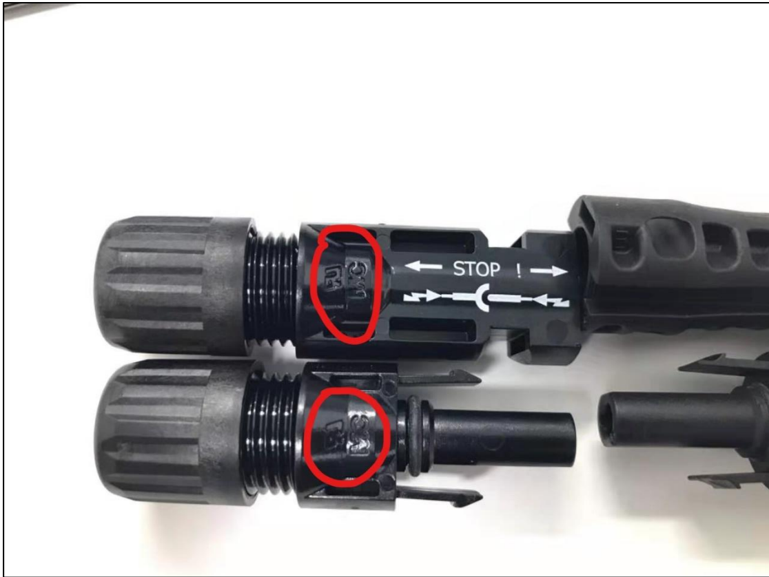
Figure 2. "MC" markings on the Staubli MC4 connector
